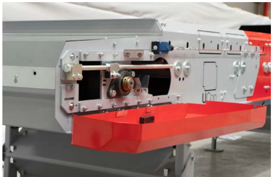
Fig. 3: When the operator pulls on the pull-wire emergency-stop, hazardous movements are safely brought to a halt.
