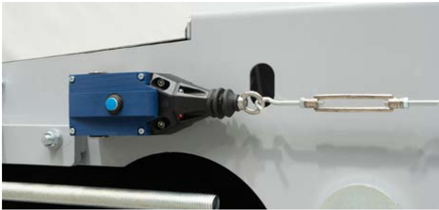
Fig. 2: The ZQ 900-22 -22 pull-wire emergency-stop from Schmersal is the integrated protective device in the WeKea modular system.
