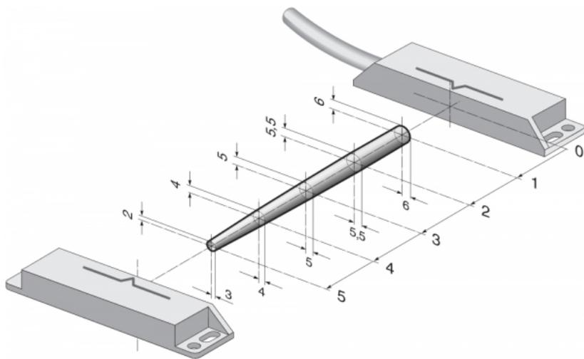
Assured switching distance:  $s_{ao}$  = 5 mm
