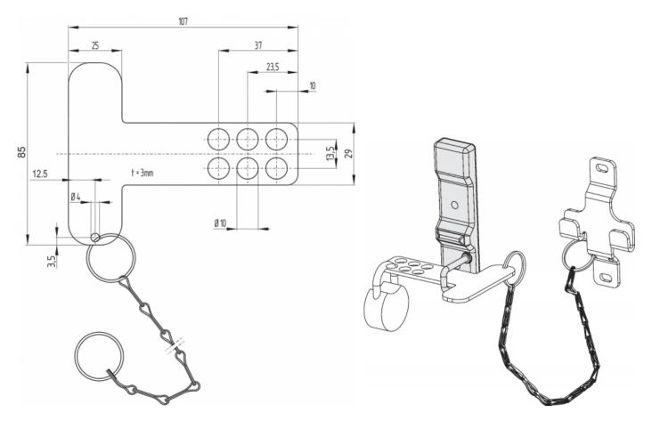
Bowden cable release ACC-AZM300-BOW-.-.M-.M (available as accessory)
