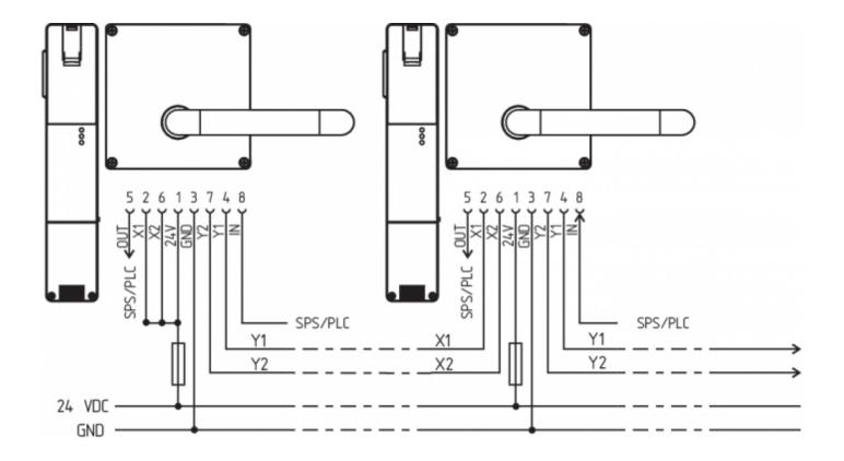
Y1 and Y2 = Safety outputs → Safety monitoring module
