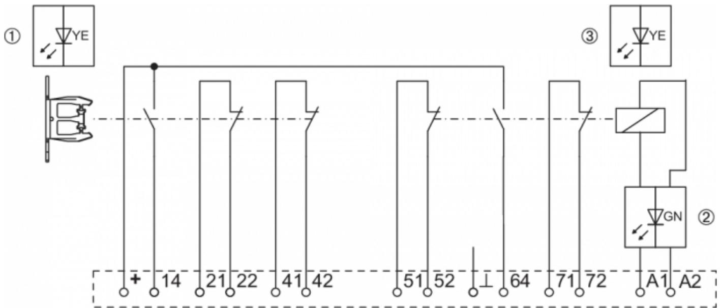
The 24 V are led internally to contacts 13 and 63. The corresponding signals of the LED display can also be tapped at terminals 14 or 64.
