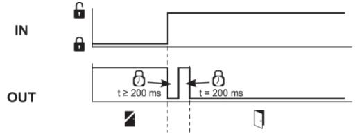
Disrupted process, door could not be unlocked
