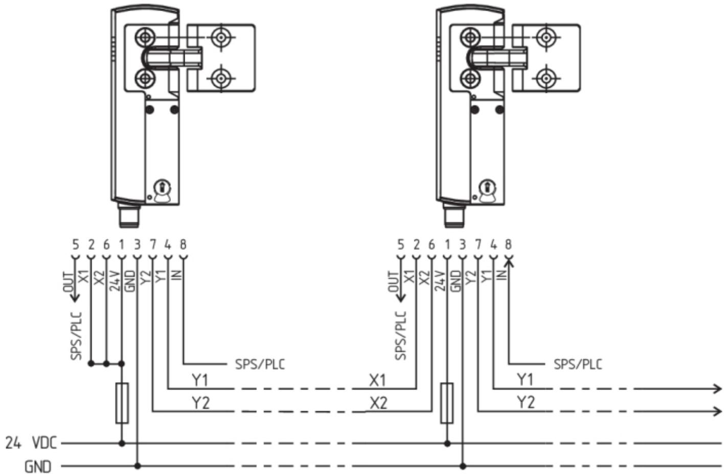
Y1 and Y2 = Safety outputs → Safety monitoring module
