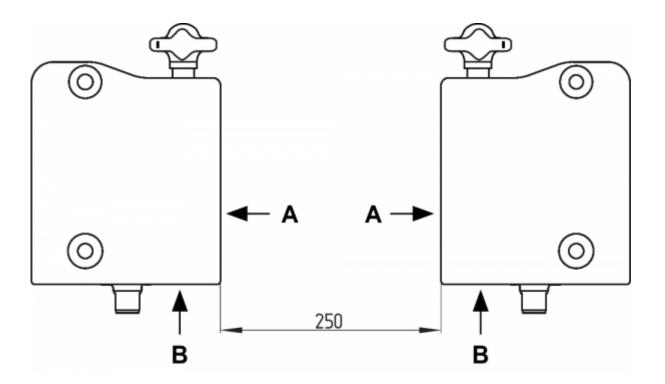
The minimum distance from metallic securing surfaces to the face side "A" and underside "B" of the device is 5 mm.
