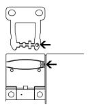
Please observe that, when fixing the switch e.g. by means of rivetting or welding, the insertion depth of the actuator is not modified. Different actuator forms are available. The actuators B1 and B5 are preferably used for sliding and removable safety guards. For hinged guards, the B6R and B6L actuators.
