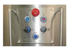
The NK cross switch, at the bottom left of the control panel, can be moved to up four positions: top, bottom, right, left.
