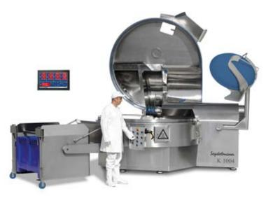
An employee operates the Seydelmann K1004 cutter. Various cross switches are available for the different functions of the machine.
