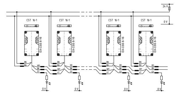
BK and RD = safety outputs Y1 and Y2  $\rightarrow$  safety-monitoring module
