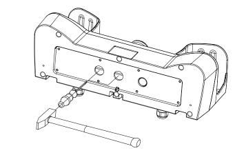
2. Route the cable through the stand and fit the two-hand control panel.
