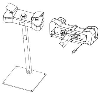
4. Open the two-hand control panel and wire the buttons. Then close the two-hand control panel again.
