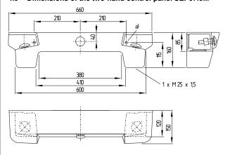
a) Mounting hole  $\varnothing$  13.5 mm Assembly on a stand is not possible.
