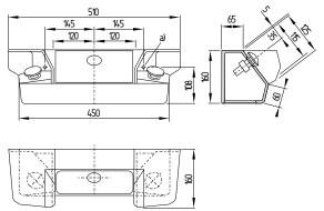
a) Mounting hole  $\varnothing$  11,5 mm Removable front plate, can be fitted with additional command devices. Holes must be made by the user.
