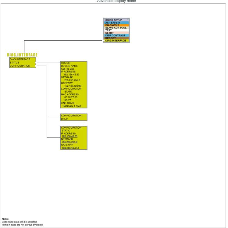
The device starts in the traditional mode. You can switch between the two modes with ESC or OK. In the advanced mode the cursor is moved by both arrow buttons. Pushing OK puts you to the superior menue (in the drawing one step to the right side). ESC puts you back to the previous menue. To edit data you first mark them with the cursor and then select them with OK, change them with the arrow buttons and finally apply them with OK. Pushing ESC cancels the editing.
