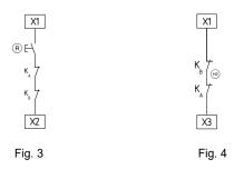
Dual-channel emergency stop circuit with command devices to EN ISO 13850 and EN 60947-5-5 (Fig. 5)
