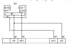
Connection of one safety edge (signal generator)
