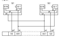
Connection of 2 safety edges (signal generators)
