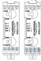
Against all other connection terminals, the safety contacts 17-18 and 27-28 comply without additional measures with the requirements for double insulation in accordance with EN 60664-1 and are to be used with switch voltages > 50 V. The safety contacts 37-38 comply with the requirements for basic insulation.
