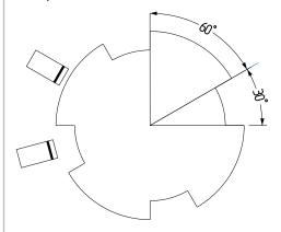
Proximity switches / pulse generators Use PNP-switching sensors with normally open function.
