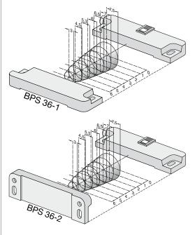
Assured switching distance:  $s_{ao} = 6 \text{ mm}$ Assured switch-off distance:  $s_{ar} = 17 \text{ mm}$
