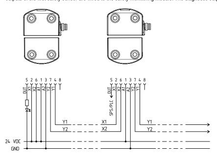
Y1 and Y2 = Safety outputs  $\rightarrow$  dual-channel safety monitoring module
