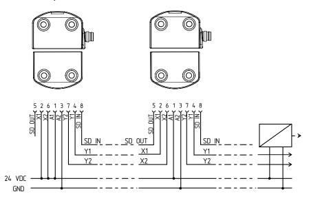
Y1 and Y2 = Safety outputs  $\to$  dual-channel safety monitoring module SD-IN  $\to$  Gateway  $\to$  Field bus
