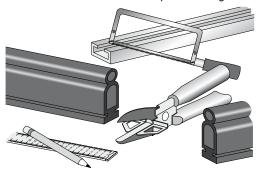
If necessary, pull the safety edge slightly out of the aluminium profile or drill mounting holes; max. hole distance 70 mm; fix the aluminium profile by means of oval-head or countersunk head screws Ø 3 ... 6 mm.
