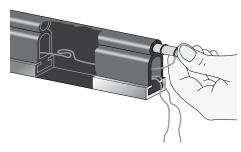
Connect the safety edge (signal generator) with the SE safetymonitoring modules after the assembly. Execute the wiring and the functional test of the safety edge in accordance with the mounting instructions SE-..C.
