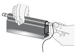
5. For the output of the connecting cables on one side, the transmitter and the receiver have different cable lengths. Pull the cable of the opposite unit through the large aperture of the rubber profile (if necessary, use the SE-WA tool). Install the end plugs.
