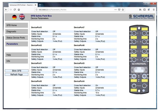
The "Parameters" page displays the set parameter values from each device port. If the SFB-PN has not been parameterized yet, the parameter values are empty!
