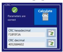
The hexadecimal CRC value can be copied via to the clipboard to be used in the engineering tool.
