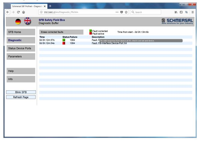
The "Diagnostics" page displays the PROFINET fault messages that the field box has sent to the PLC.
