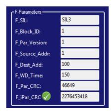
The SFB Configuration Tool compares the calculated CRC values and the values transmitted by the F-PLC.
