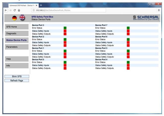
The "Status Device Ports" page displays the fault status and I/O status of each device port.
