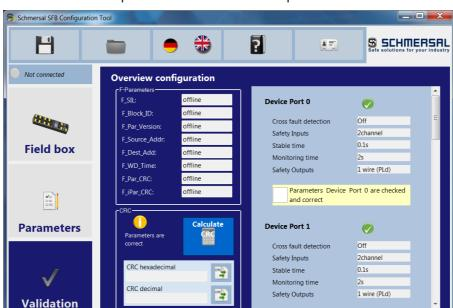
2. Validation of the parameters for each device port
