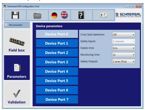
Enter the device parameters for each device port and note the dependencies between the parameters. The optimal parameters for the different device types can be found in Chapter 2.3 "Wiring examples and parameterization".
