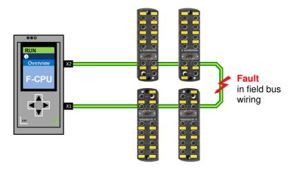
The function of a Media Redundancy Manager (MRM) consists in checking the ring structure required by the configuration for its operability. This is done by sending cyclic test telegrams. As long as the test telegrams are received again by the MRM, the ring structure is intact. An MRM uses this behaviour to prevent circulation of telegrams and to convert a ring structure into a line structure.
