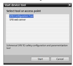
With TCI support, the default parameter settings are transferred to the SFB Configuration Tool when it is started.
