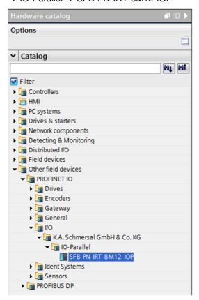
With "Drag & Drop" you can insert the SFB-PN in the window "Devices & networks".
