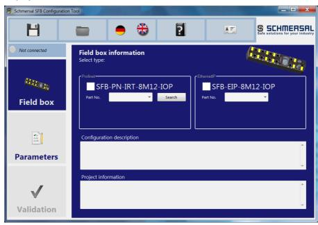
Select the field box variant SFB-PN-IRT-8M12-IOP with the checkbox. The corresponding part number is displayed.
