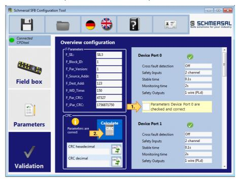
With the checkbox (1.) you confirm that the parameters for each device port X0 - X7 have been checked.
