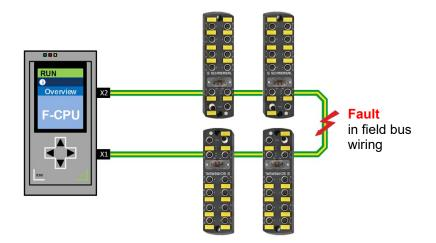
The function of a Media Redundancy Manager (MRM) consists in checking the ring structure required by the configuration for its operability. This is done by sending cyclic test telegrams. As long as the test telegrams are received again by the MRM, the ring structure is intact. An MRM uses this behaviour to prevent circulation of telegrams and to convert a ring structure into a line structure.
