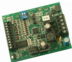
Figure 15: Board CAP-02 for connecting the landing calls to the CANopen lift bus
