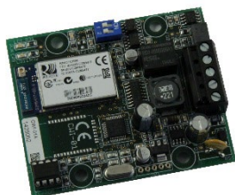
Figure 17: Board CWI-01 for remote control of the control system (e.g. from the car) using a mobile device (phone, tablet, notebook).
