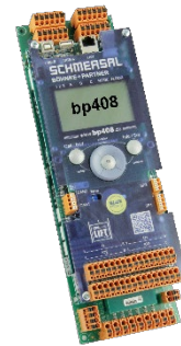
Figure 11: The control system bp408 is equipped with all the modern interfaces of lift technology
