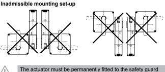
and protected against displacement by suitable measures (tamperproof screws, gluing, drilling of the screw heads, pinning).
