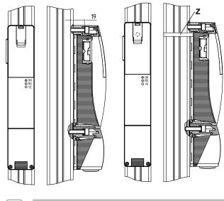
Mounting tolerance - horizontal: ± 2.5 mm
