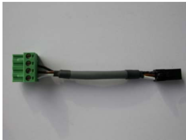
Figure 4-6 SN-I/F communication cable
