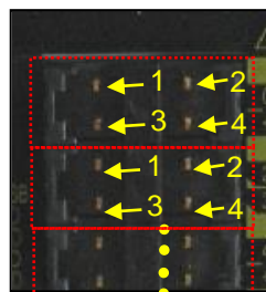
Figure 3-33 PSC-S-IN-E terminal diagram
