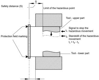
≤ 75 mm = max. distance for protection against stepping over To prevent persons from stepping over the protection field this dimension must be imperatively respected and observed.
