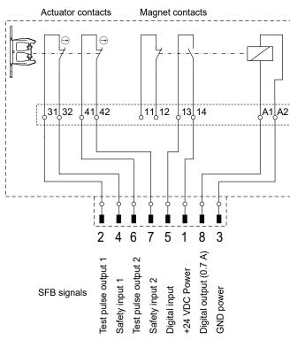
Signal pin 5 "safety guard unlocked"
