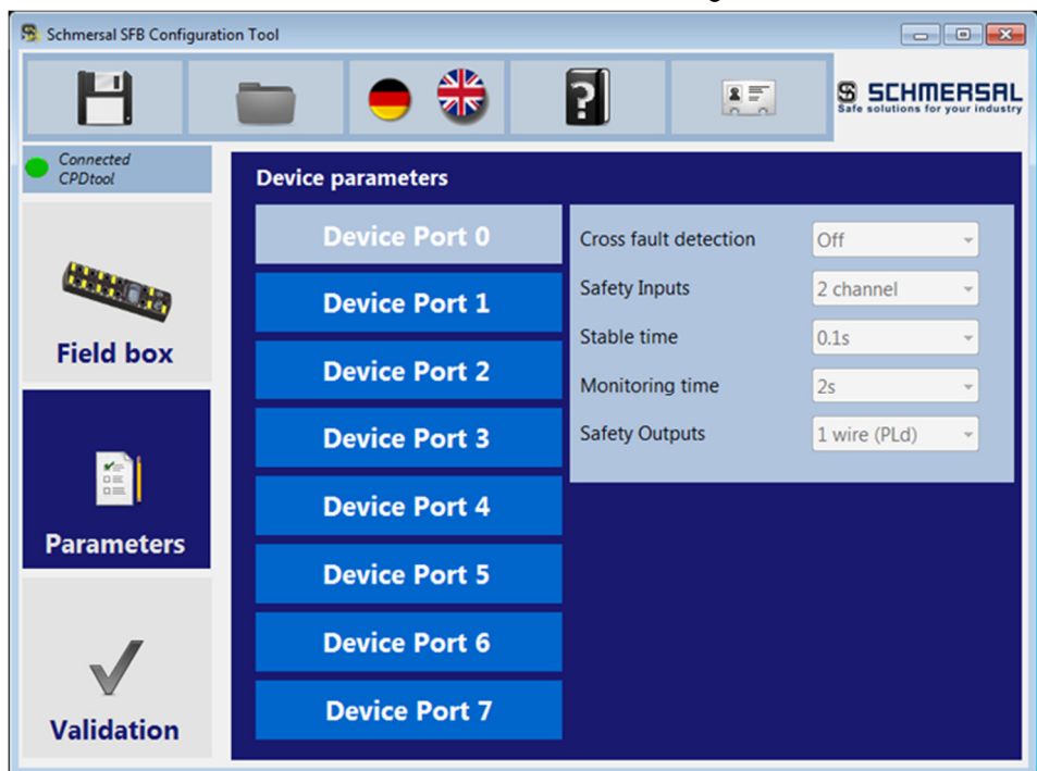
Figure 15: transferred parameters from the engineering tool
