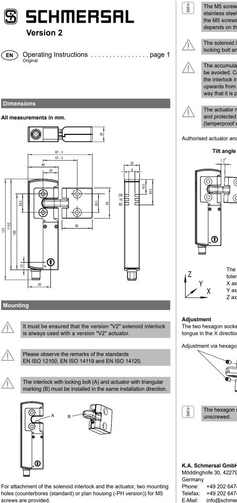
The M5 screws must be at least strength class 8.8 or, in stainless steel, strength class 80. The tightening torque of the M5 screws is 4 ... 6 Nm, the maximum tightening torque depends on the fastening screws used.
