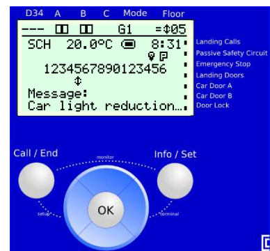
Figure 27: Display and keys of bp308. Here is a display of two doors A and B.
