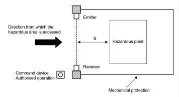
The formulas and calculation examples are related to the vertical set-up (refer to drawing) of the safety light grid with regard to the hazardous point. Please observe the applicable harmonised EN standards and possible applicable national regulations.
