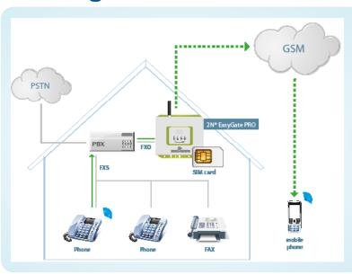
In this scenario, companies connect the  $2N^{\oplus}$  EasyGate PRO to their existing PBX with an analogue interface. All calls to mobile networks are routed via the gateway and customers can save up to 70 percent on their calling costs.
