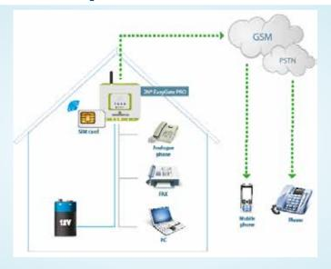
You can connect an analogue phone or PBX to get voice connection. A PC connected to a USB port can access the Internet and send/receive SMS messages.
