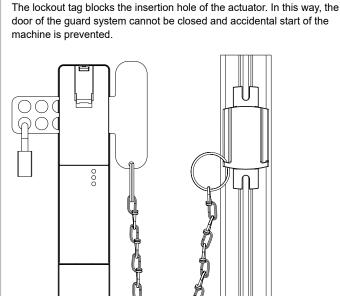
Usage of SZ201-1 with safety switch AZ201 or solenoid interlock
