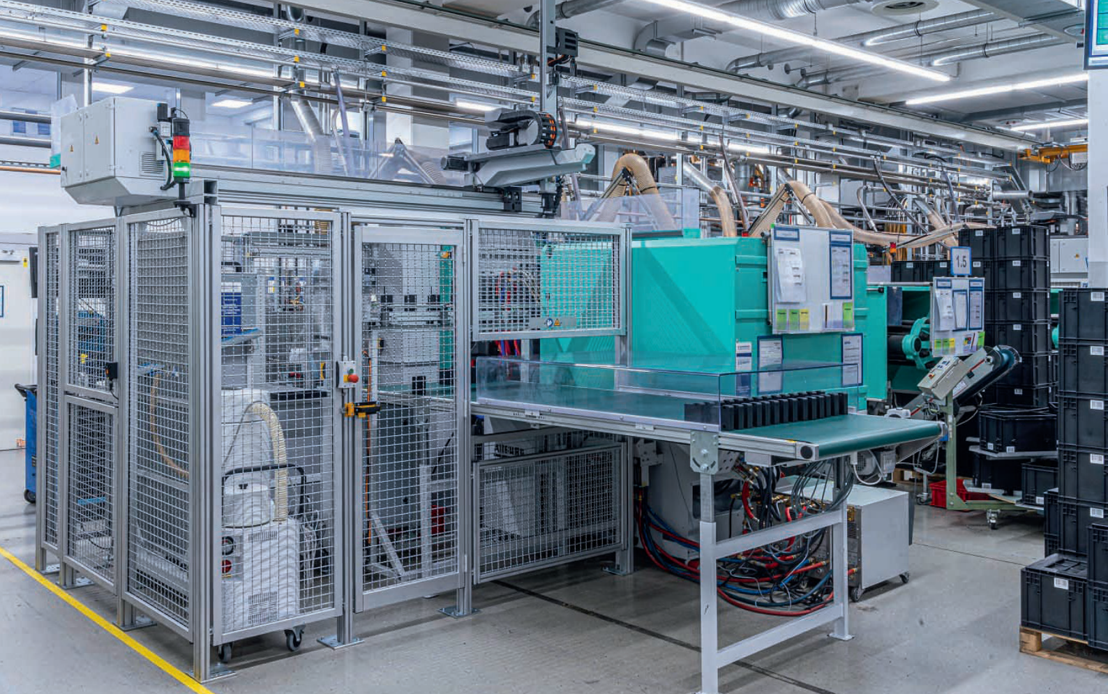
Many Schmersal switches are manufactured using the injection moulding process.
