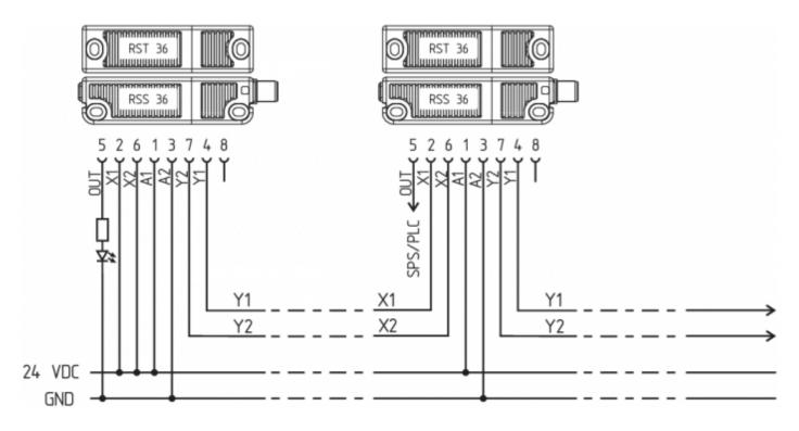
Y1 and Y2 = Safety outputs  $\rightarrow$  Safety monitoring module
