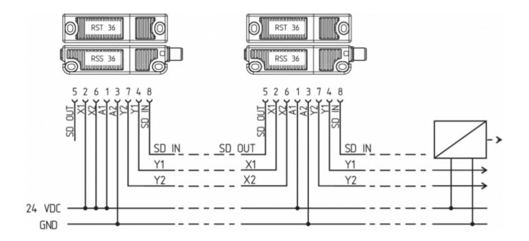
Y1 and Y2 = Safety outputs  $\rightarrow$  Safety monitoring module SD-IN  $\rightarrow$  Gateway  $\rightarrow$  Field bus
