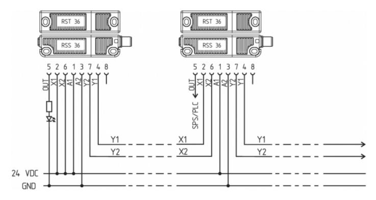
Y1 and Y2 = Safety outputs  $\rightarrow$  Safety monitoring module
